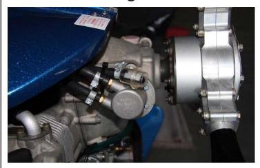
Gordon Douglas of East of Scotland Microlights has come up with a clever idea to stop bugs crawling up the vent pipe of his Rotax 912's fuel pump. Told about it by a French engineer at Montpezat, Gordon uses a standard nylon mesh fuel filter cut open at one end to stop large bugs crawling up the pipe to block it. Gordon wasnt sure if Scotland has big enough bugs to do that, but thought it was a good option for flying in France.
